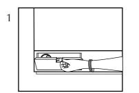
Open the bottom door, which is detachable by pressing the top portion of it.
